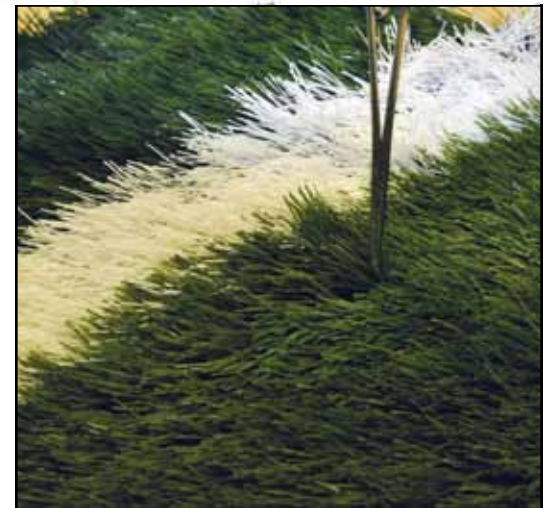
Each roll of turf is tested to ensure the required 9 lb tuft bind
