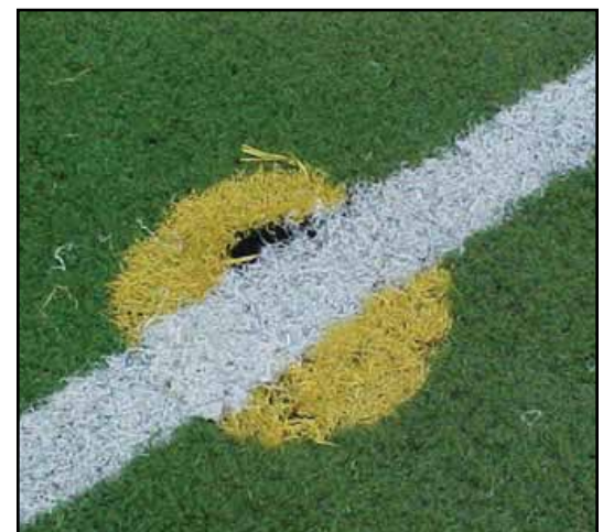
Other systems like the one shown here typically average in the neighborhood of 5- 7 lbs/force on their tuft bind tests
